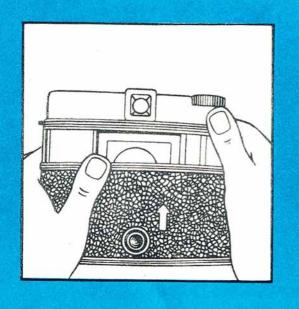
To close the camera put the back cover in position and turn the catch at the bottom to the word "LOCK".
