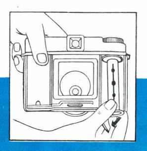
Put the empty spool in the upper spool chamber and swing out the lower spool holder. Put the film in the lower spool chamber with the tapered end of the backing paper towards the empty spool, then swing the spool holder back into the spool chamber.
