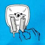
ATTACH TO CAMERA—Flash gun is installed by pushing flash gun pins into recentacles on camera.
